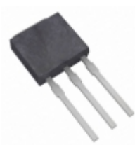
L4006V6 Littelfuse Inc. TRIAC SENS GATE 400V 6A TO251
