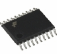
74LVT573MTCX Fairchild/ON Semiconductor IC LATCH TRANSP OCT 3ST 20TSSOP
