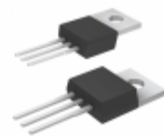
IXTP12N50P IXYS MOSFET N-CH 500V 12A TO-220
