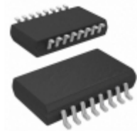
ADUM3401TRWZ-EP-RL Analog Devices Inc. DGTL ISO 2.5KV GEN PURP 16SOIC
