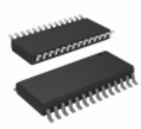
MCP23016T-I/SO Micrel / Microchip Technology IC I/O EXPANDER I2C 16B 28SOIC
