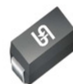
RS2DAH2G TSC (Taiwan Semiconductor) DIODE GEN PURP 200V 1.5A DO214AC
