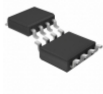
LTC4441ES8-1#PBF ADI (Analog Devices, Inc.) IC MOSFET DRIVER N-CH 8-SOIC
