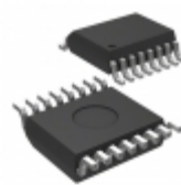
MIC9130BQS Microchip Technology IC CTRLR DC-DC PWM HV HS 16-QSOP
