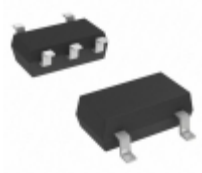
XP0111500L Panasonic Electronic Components TRANS PREBIAS DUAL PNP SMINI5
