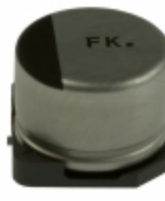
EEV-FK1K100P Panasonic Electronic Components CAP ALUM 10UF 20% 80V SMD
