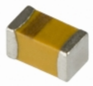
TACL475M004R AVX Corporation CAP TANT 4.7UF 4V 20% 0603
