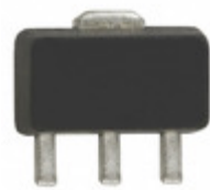
RF33375TR7 RFMD IC AMP HBT GAAS GEN-PUR SOT-89
