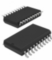
74LVQ374SJX AMI Semiconductor / ON Semiconductor IC FF D-TYPE SNGL 8BIT 20SOP
