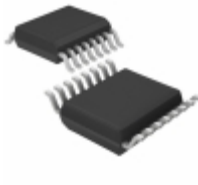
ADN4667ARUZ-REEL7 ADI (Analog Devices, Inc.) IC DRIVER DIFF LVDS 4CH 16TSSOP
