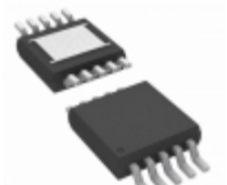
LTC1403ACMSE#TRPBF Linear Technology IC ADC 14BIT 2.8MSPS DIFF 10MSOP
