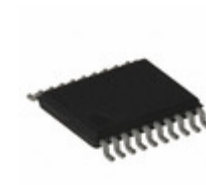
ATF16V8CZ-12XC Microchip Technology IC PLD 8MC 12NS 20TSSOP
