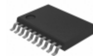
QS3VH244PAG8 IDT, Integrated Device Technology Inc IC BUS SWITCH 8BIT QUICK 20TSSOP
