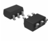
XN0411500L Panasonic Electronic Components TRANS PREBIAS DUAL PNP MINI6
