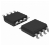
PIC12F609T-I/SN Microchip Technology IC MCU 8BIT 1.75KB FLASH 8SOIC
