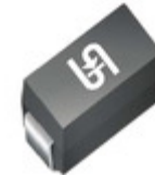
1SMA5940HR3G TSC (Taiwan Semiconductor) DIODE ZENER 43V 1.5W DO214AC
