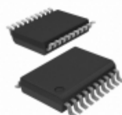
ADG467BRSZ Analog Devices Inc. IC CHAN PROTECTOR OCTAL 20-SSOP
