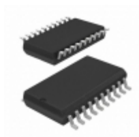
AT90S2313-4SC Microchip Technology IC MCU 8BIT 2KB FLASH 20SOIC
