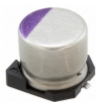
16SVPC68M Panasonic Electronic Components CAP ALUM POLY 68UF 20% 16V SMD
