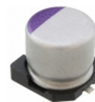
16SVPF180M Panasonic Electronic Components CAP ALUM POLY 180UF 20% 16V SMD
