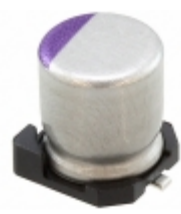
2R5SVPE330M Panasonic Electronic Components CAP ALUM POLY 330UF 20% 2.5V SMD
