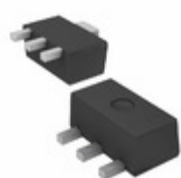
AP2138R-1.8TRG1 Diodes Incorporated IC REG LDO 1.8V 0.25A SOT89
