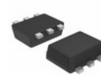
EMZ1DXV6T1 ON Semiconductor TRANS NPN/PNP 60V 0.1A SOT563
