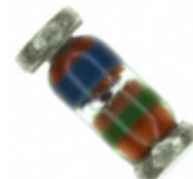
FLZ4V3B Fairchild/ON Semiconductor DIODE ZENER 4.3V 500MW SOD80
