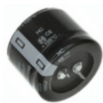
EET-HC2W391LA Panasonic Electronic Components CAP ALUM 390UF 20% 450V SNAP
