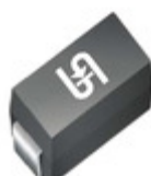
1SMA4746HM2G TSC (Taiwan Semiconductor) DIODE ZENER 18V 1.25W DO214AC
