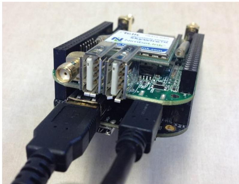
Figure 2-2 Cape to Beaglebone USB Connection
