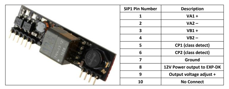
R21 controls the PoE class that is seen by the power source. By default this is set to class 0, the most flexible option in the original PoE spec. R18 and R20 can be loaded to adjust the 12V output. See the AG9120-S datasheet for details. Note that most uEZGUIs average around 1W-3W power draw, so class 1 or class 2 would be suitable for most uEZGUI final hardware implementations (such as an access control box) without additional power loads.
