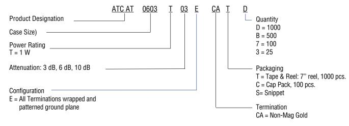
The above part number refers to an ATC AT 0603 Case Size with an attenuation of 3dB, 1W Power Rating, wrapped and patterned ground plane configuration with Non-Mag Gold Termination and tape and reel packaging, 1000 pcs.
