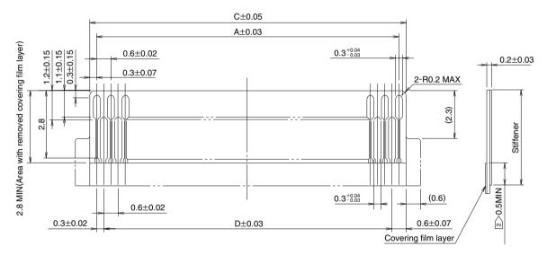
1 Polyamide and thermally hardening adhesive is recommended as the stiffener materials.
