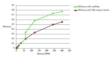
Figure 4: Energy Efficiency Example with coolStep
