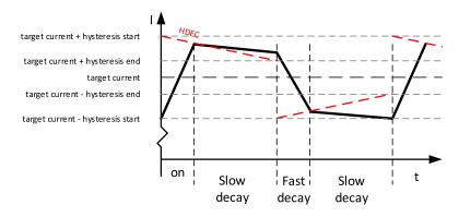
Figure 2: spreadCycle principle
