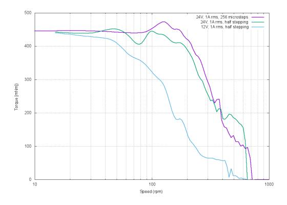
Figure 10: PD42-3-1270 torque vs. speed
