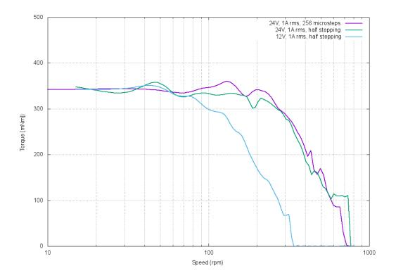
Figure 9: PD42-2-1270 torque vs. speed
