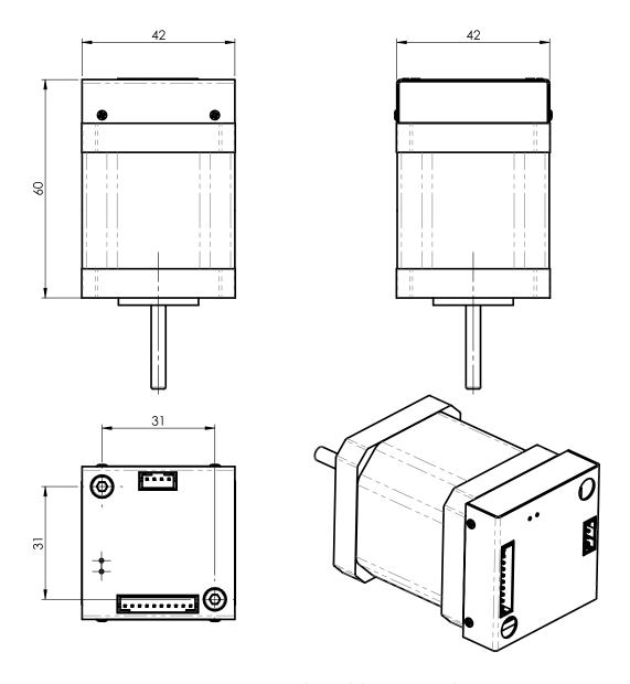
Figure 7: PD42-3-1270 mechanical dimensions with motor
