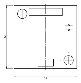
Figure 6: PD42-1270 top view mechanical dimensions
