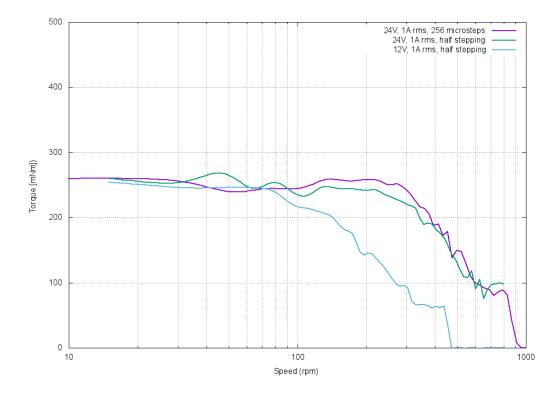
Figure 8: PD42-1-1270 torque vs. speed
