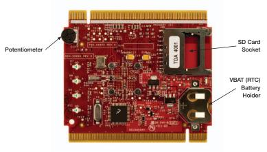
Figure 2: Back side of TWR-K60D100M module.
