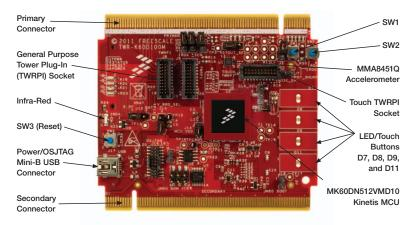
Figure 1: Front side of TWR-K60D100M module.
