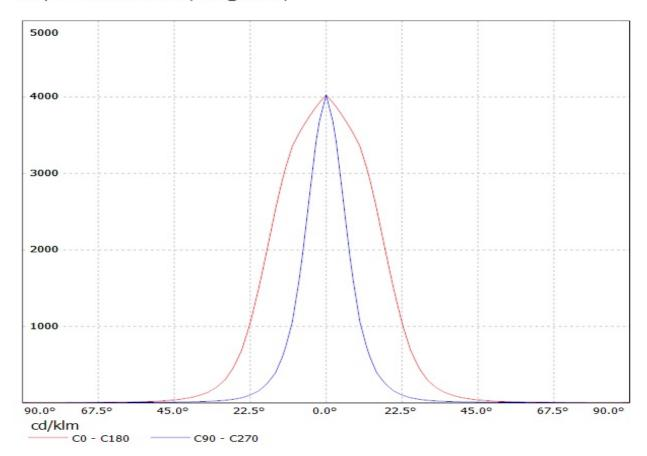
Luminaire: LEDIL OY CP12673\_TINA2-O (XB-D) Efficiency=84% Lamps: 1 x Cree XB-D white (97lm @ 250mA)
