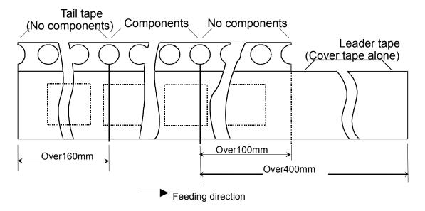
6) The tape for chips are wound clockwise, the feeding holes to the right side as the tape is pulled toward the user.
