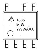
First and Second Lines: Logo and Marking ID Third Line: Date Code Y: Year WW: Work Week of Molding A: Assembly House Code XX: 7<sup>th</sup> and 8<sup>th</sup> Digits of Batch No.
