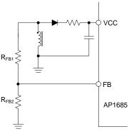
Figure 3. OVP Circuit
