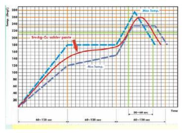
Fig 2. Infrared soldering profile
