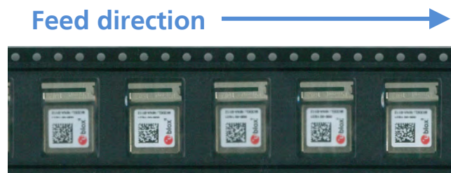
Figure 13: Orientation of NINA-B112 modules on tape
