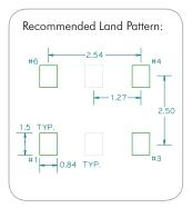
\*Note: pads 2 and 5 are optional (shown as dotted lines). XO's are designed to fit on industry standard, 4 pad layouts.
