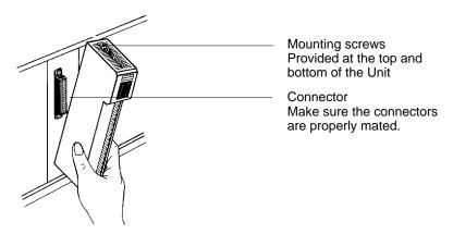
The figure below shows one I/O Unit mounted directly to the left slot of the CPU Rack.
