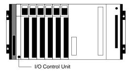
Now we can use a cable to connect the CPU Rack to another Backplane. This Backplane has a Power Supply and I/O Units mounted to it, but it has no CPU of its own. The additional Backplane must also have an I/O Interface Unit mounted to its leftmost position. This configuration of additional Backplane, Power Supply, I/O Units, and I/O Interface Unit is called an Expansion I/O Rack.
