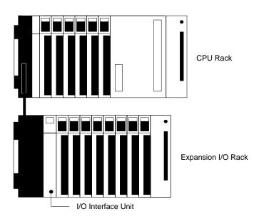
The CPU Rack and Expansion I/O Rack shown above are connected by a cable. Remember that this whole configuration is still referred to as one PC. It is possible to keep adding Expansion I/O Racks in this way until the maximum number of I/O points for the system is reached. Each Expansion I/O Rack needs an I/O Interface Unit.
