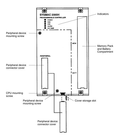
Peripheral Device Connector The CPU is equipped with one connector for peripheral devices. A peripheral device, such as the CPU-Mounting Programming Console, can be mounted directly to the CPU and does not require a connecting cable. To mount the CPU-Mounting Programming Console or any other peripheral device directly to the CPU, follow these steps:
