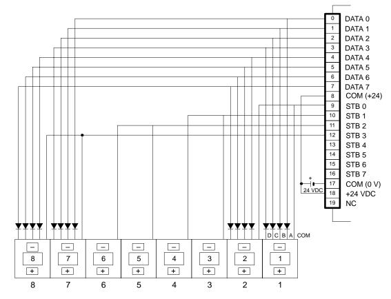
The table below shows the combinations made possible when the digital switches are wired as shown in the figure above.
