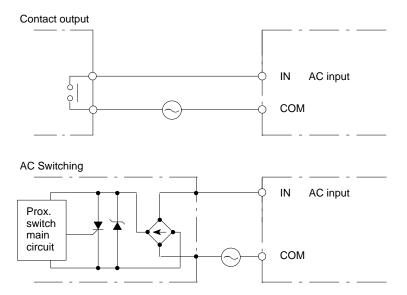
**Note** If a reed switch is used as the input contact of the AC Input Unit, the reed switch must have a permissible current capacity of 1 A minimum, otherwise contact weld may result due to inrush current.
